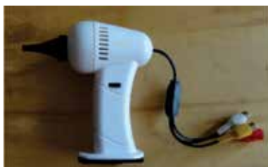
Figure 6. Side view of the low-cost, custom-made video-otoscope.
